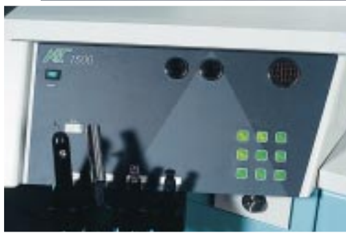
Main control display featuring nine function switches and four instrumentholders (three of them switchable)
